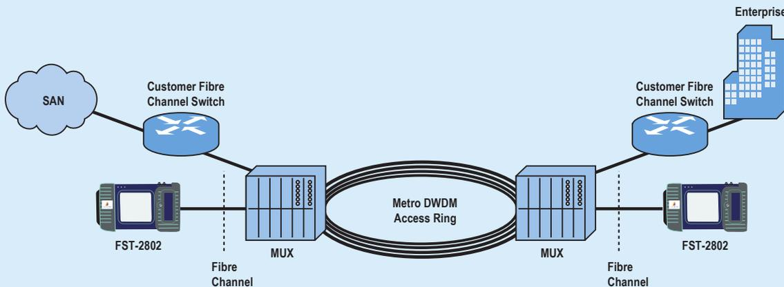
Diagram 1. Fibre Channel Testing on Metro DWDM Network
