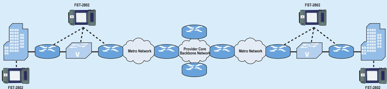
Diagram 2. IP Traffic Testing in Metro Networks
