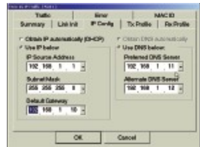
Figure 6. Configuration Page for Source IP Address
