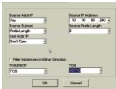
Figure 5. Receive Profile Page for IP Traffic
